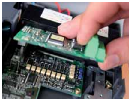
Connector system for time-saving installation
